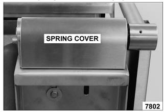
3. Place a 1 5/8" wrench on the lid spring lock nut and apply a downward force until locking pin can be removed. Continue to hold lock nut in place.
